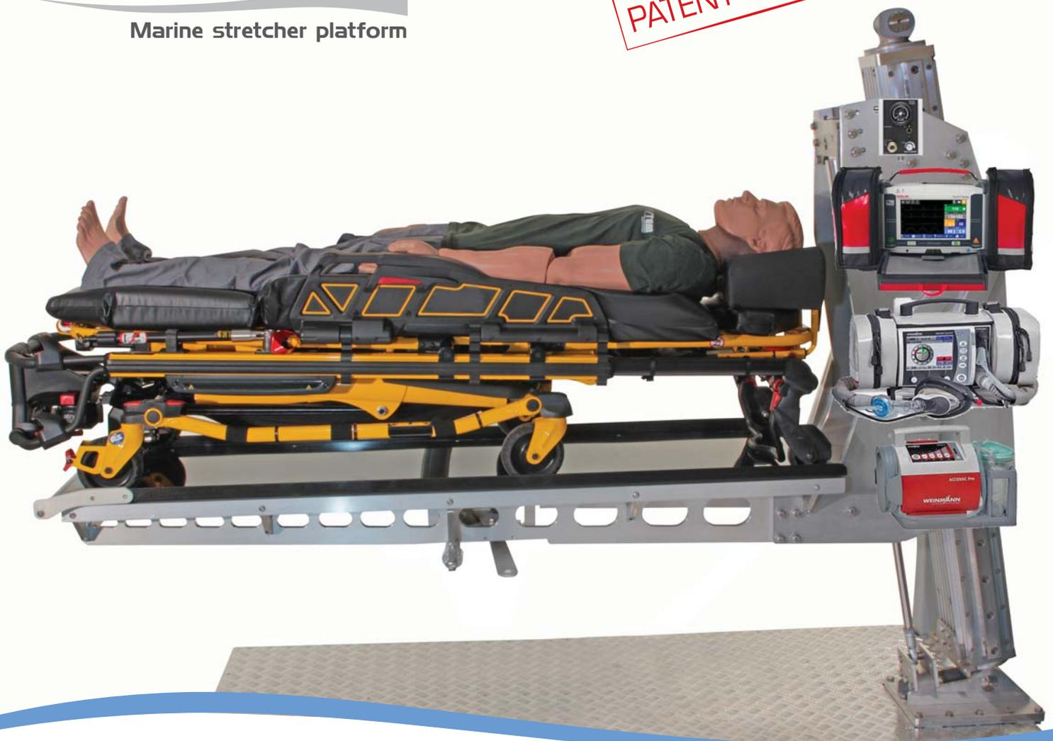
Shock-absorbing support for nautical-use stretchers, with self-adjusting hydro pneumatic suspension based on the patient's weight. Particularly recommended for high-speed boats, it can absorb shocks due to the impact with the waves with values up to 10 g.
